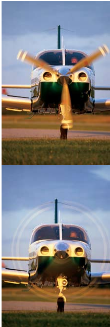
Paint bands on propellers and rotor blades become visible concentric circles when in motion, helping ground personnel identify and avoid their dangerous arcs.
