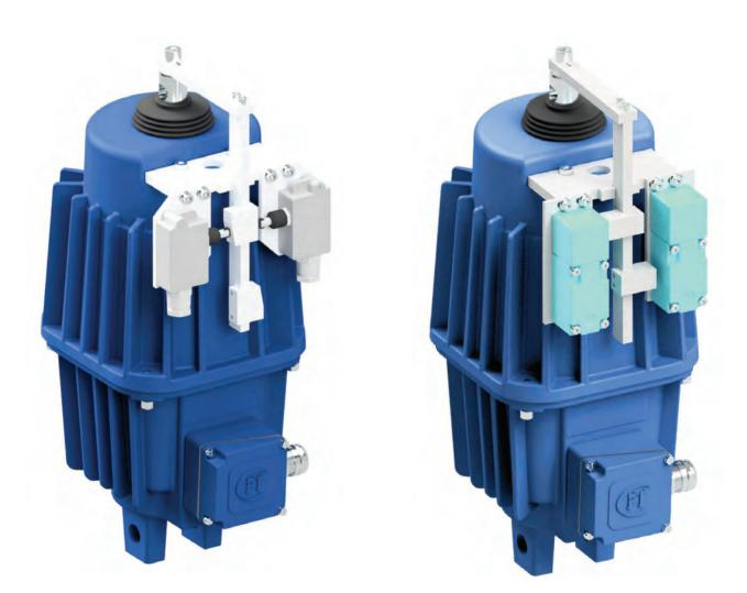
Microswitch is build on the outside of cylinder. It is activate when the piston is in the top position. In a magnetic inductive switch, switches are also built on the outside of the cylinder and activates them a permanent magnet built in the piston. The advantage of this solution is that the switches are fully protected from external influences and in this way are very reliable in the work. Linkage is done in connecting box.
