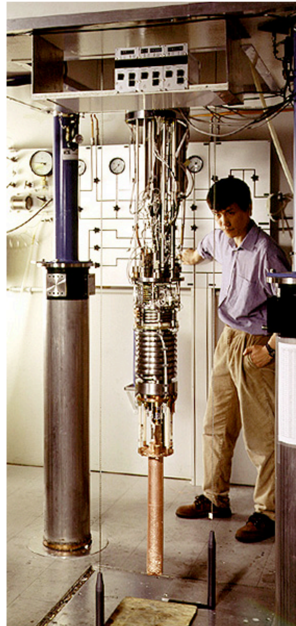
The new microkelvin refrigerator became operational in 1998. It provides a platform for ultralow temperature experiments below 100 microkelvin in high magnetic fields up to 7 T. In 1999, the nuclei of a single crystal rhodium sample were cooled in this apparatus to the record breaking temperature of 250 picokelvin.
