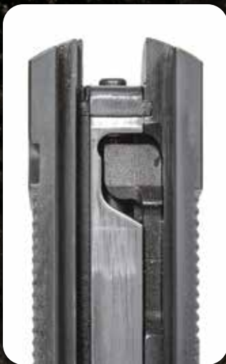
Left: The Girsan comes with the Devel-designed firing pin safety that appeared on MkIIIS Hi-Powers. It is the most seamlessly integrated such safety Jeremy has ever seen.
