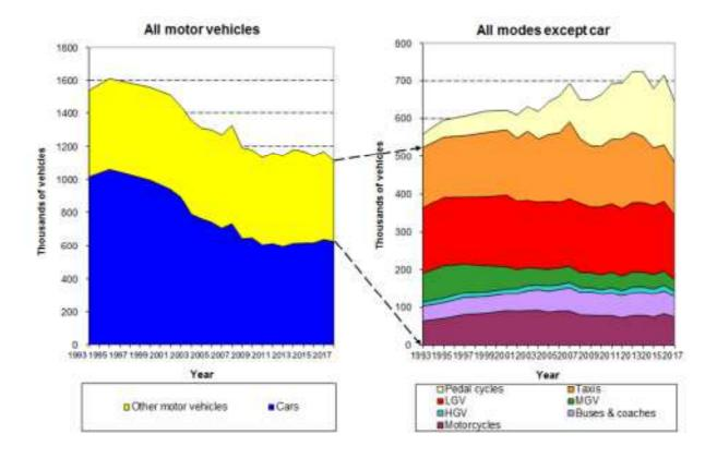
Figure 4 – Combined direction all day traffic crossing the Central Cordon by vehicle type, 1993 to 2017
