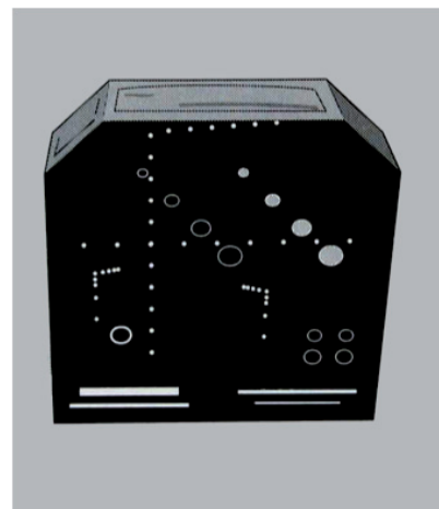
Figure 23. A tissue-mimicking phantom
