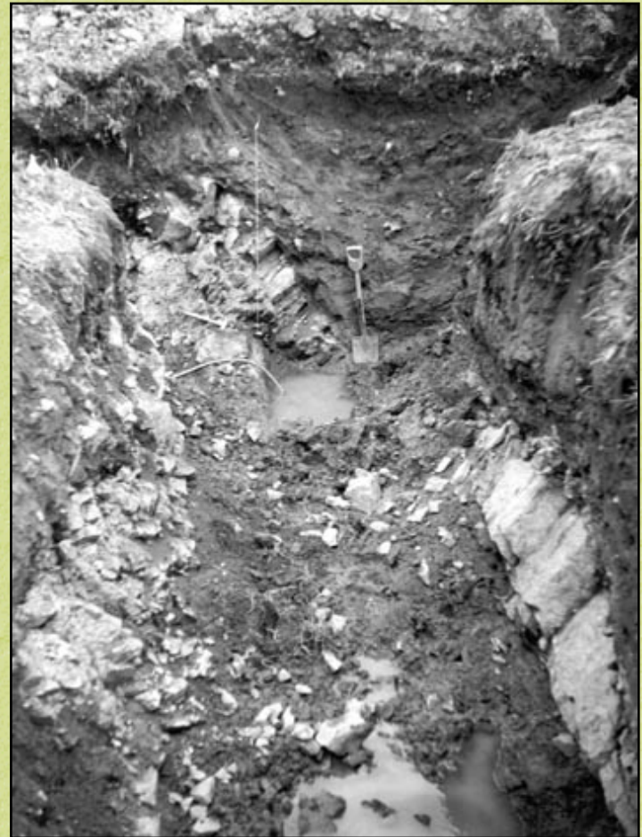
Above: Photograph of one of the trenches dug in 1963 showing a chert bed dipping steeply to the northeast (to the right in photograph).
