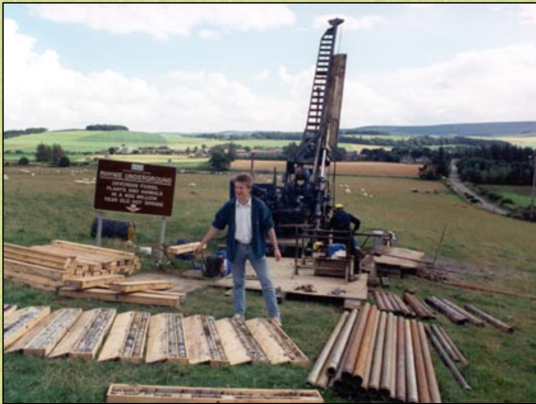
Above: Cores of the Rhynie sequence recovered by drilling have been carefully marked and transferred into core boxes for storage and study back in the lab.
