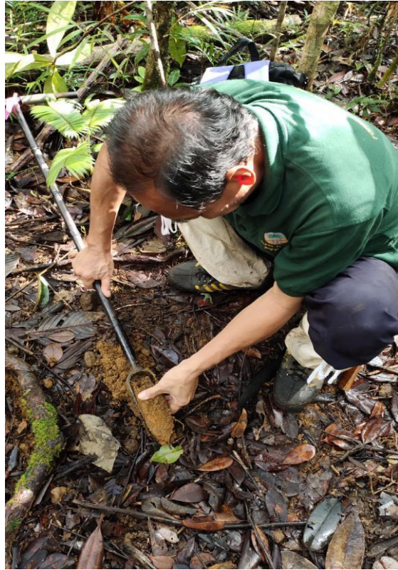
Figure 11. Arranging the soil sample in horizontal position.
