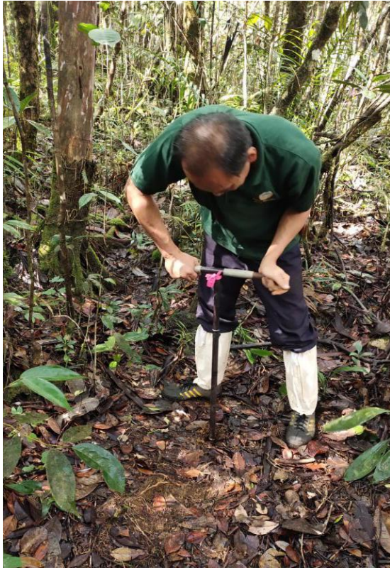
Figure 10. Taking sample with soil auger.
