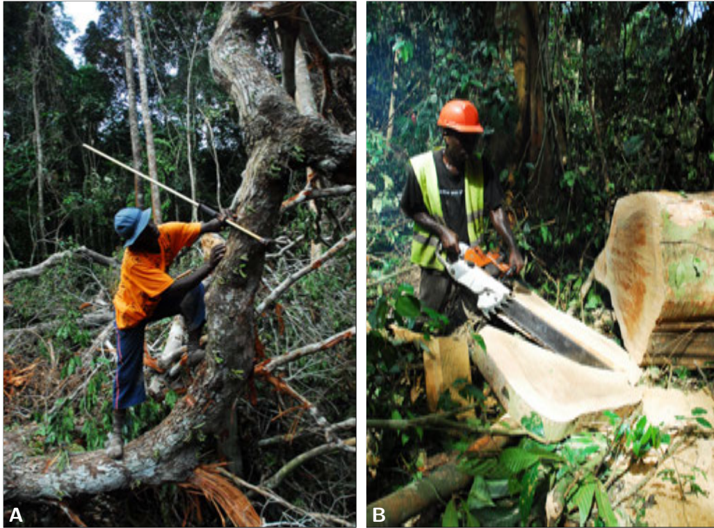
PHOTO 3.10 – Measuring a large tree in the field: (A) measuring the volume of a tree of diameter > 20 cm, (B) taking aliquots of wood from the trunk (photos: M. Henry).
