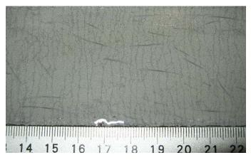
Figure 2. Distinctive fine multiple cracking upon strain hardening of UHP-FRC with only 1.5 % twisted high strength steel fibers.
