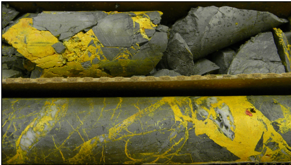
Orpiment and realgar breccia in a drill core, Twin Creeks mine, Nevada.
