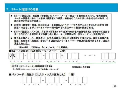
Figure 4. B-route authentication ID and password contents allocated by power company, etc.,
