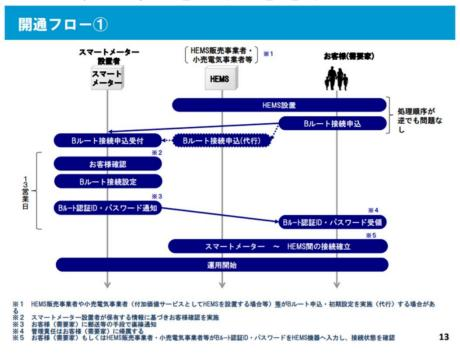
Figure 3. Basic operating flow of smart meter B-route: at opening
