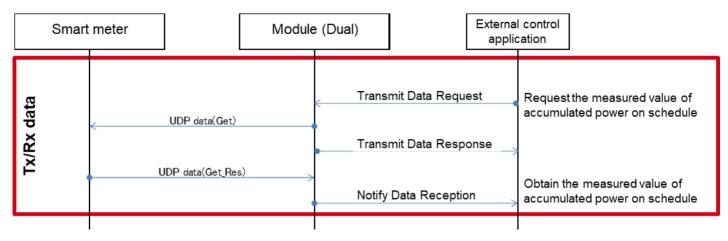
Figure 7. B-route data Send/Receive sequence
