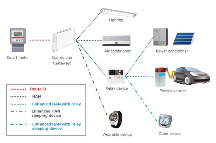
Figure 1. Network Configuration Example
