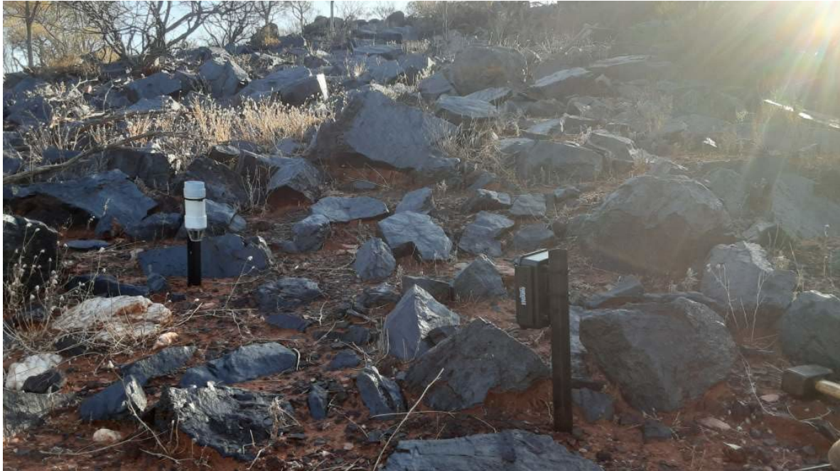
Plate 1. An example of a camera trap setup in Rocky Mulga Shrubland in the survey area (camera is in the foreground and the bait station in the background).
