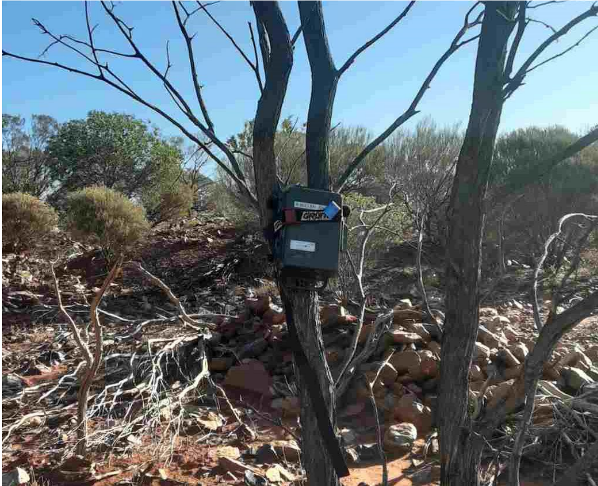
Plate 2. Example of an SM4 setup in the survey area to detect the calls of the Night Parrot.
