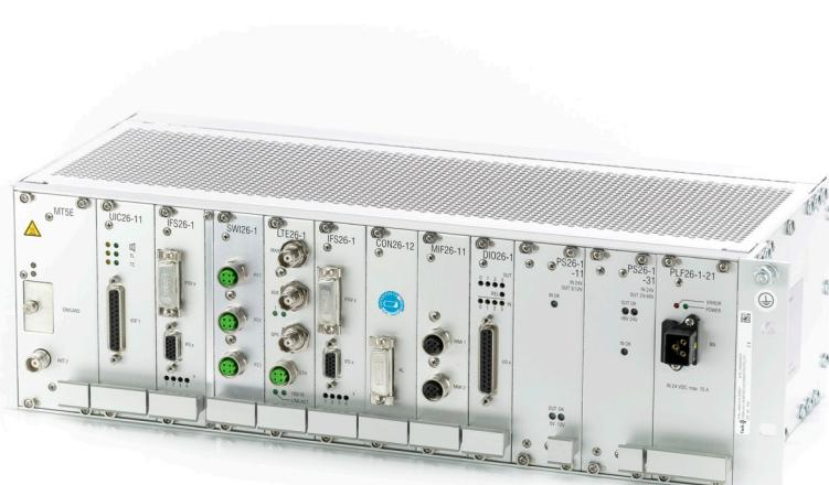
The CR26 central unit is a train radio for GSM-R radio networks and ensures the operational communication of the train driver. The CR26 can be extended with an ARM26/ARM26C analog radio to a dual-mode train radio for voice radio/shunting radio and data radio applications.
