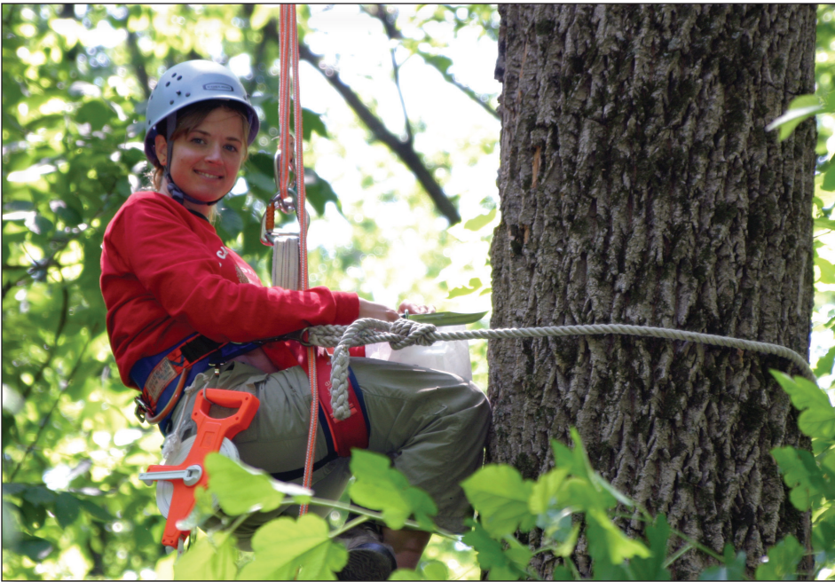
Figure 31. Courtney Kilgore collecting tree bark samples for corticolous myxomycetes cultured in moist chambers. Notice the reel-bound tape to measure height of bark sample, the climbing saddle attached to a climbing rope, and a much stronger, thicker safety rope secured around the tree trunk so that both hands are free to collect specimens.
