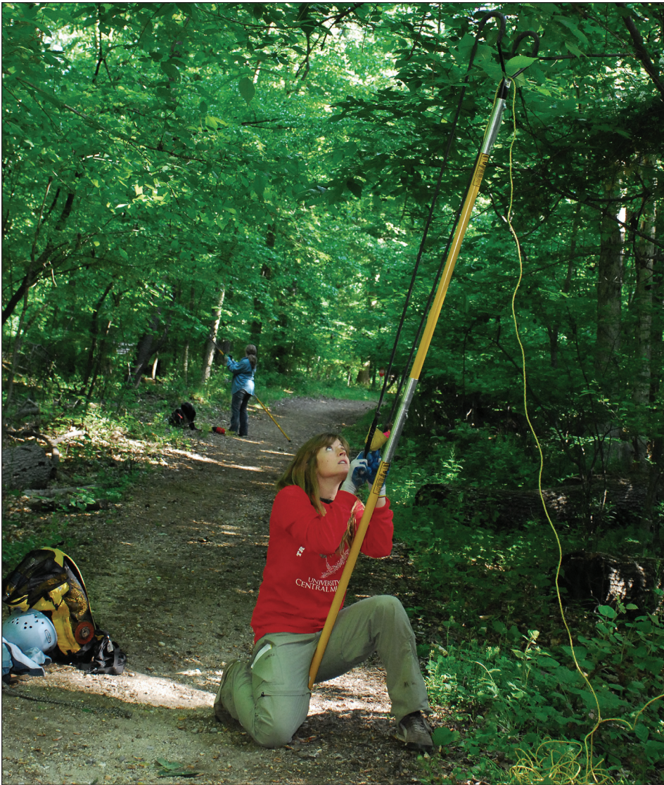
Figure 29. The Doubled Rope Climbing Method. Ready, set, shoot! The Big Shot sling shot enables the shooter to accurately direct a throw bag attached to a throw line 70–80 ft over a sturdy tree limb or preferably a tree crotch.
