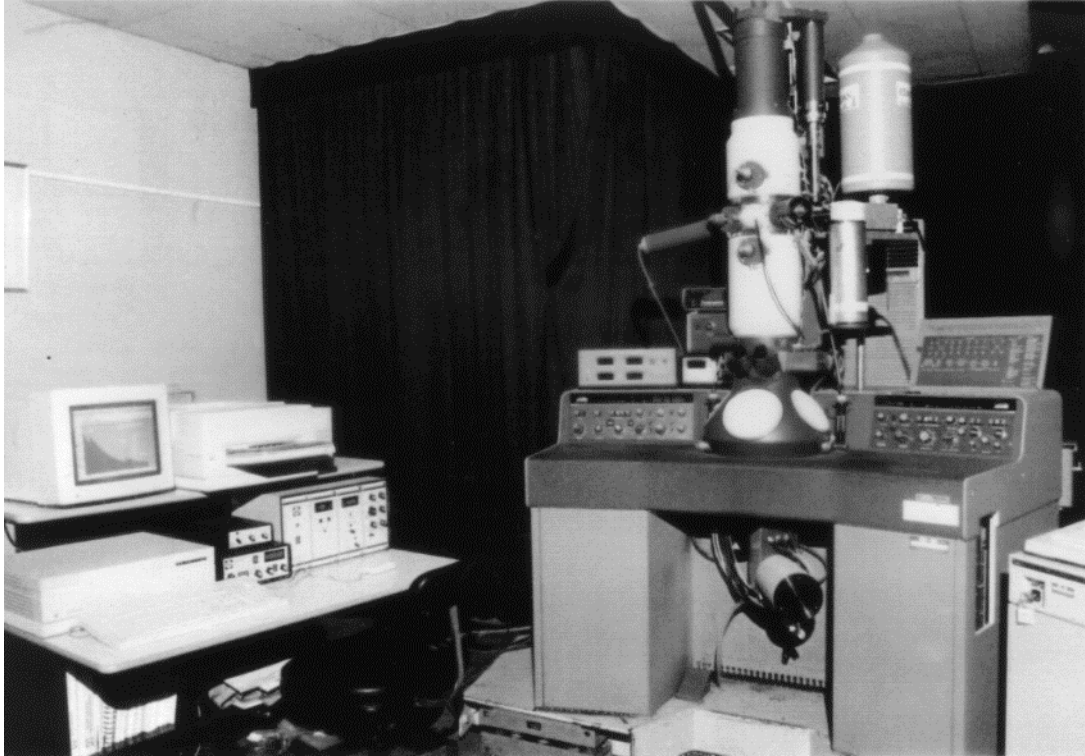
Transmission electron microscope with electron energy loss spectrometer below column and control electronics on desk to left.
