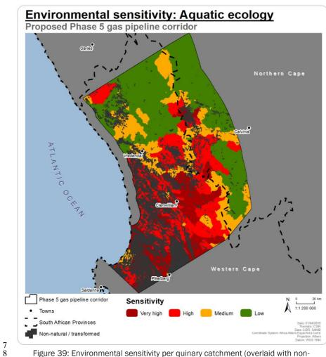
Figure 39: Environmental sensitivity per quinary catchment (overlaid with nonnatural/transformed landcover) of aquatic ecosystems to proposed gas pipeline development in the Phase 5 corridor.
