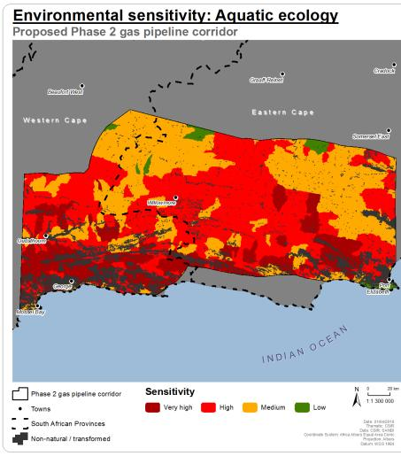
Figure 45: Environmental sensitivity per quinary catchment (overlaid with nonnatural/transformed landcover) of aquatic ecosystems to proposed gas pipeline development in the Phase 2 corridor.
