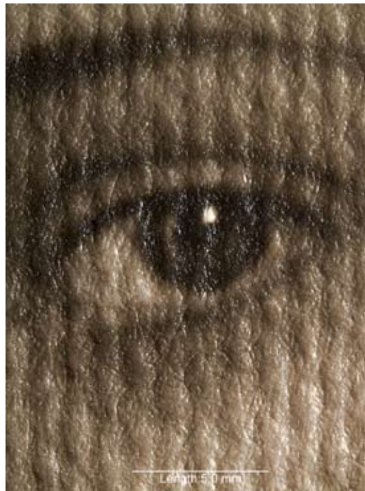
Kodak Opal Grade Z [Tapestry] photographic paper sample and micrograph. "Photographic Papers Manufactured By Eastman Kodak Company" Rochester, Eastman Kodak Company., circa 1937 10.7 x 16.2 cm.
