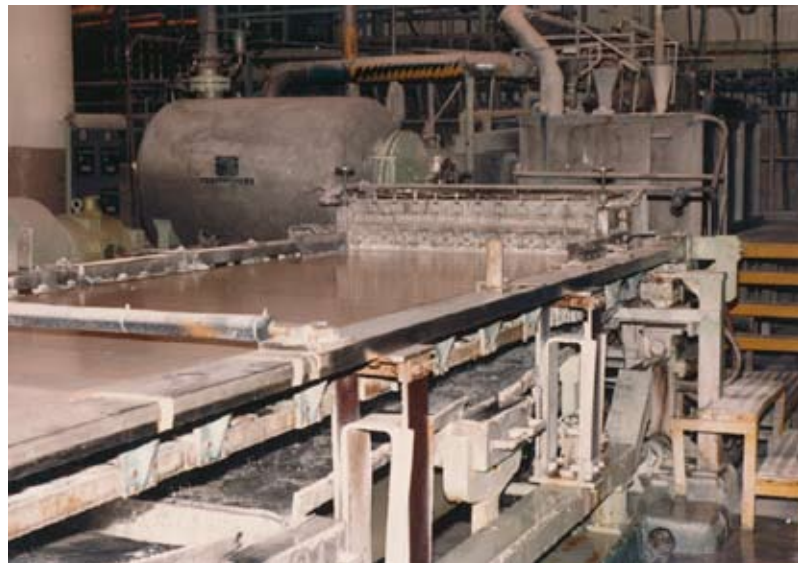
(Fig. 2.2) The forming section of a 50-inch (wide) Kodak papermachine (1986). The pulp/water mixture is moving toward the camera position.
