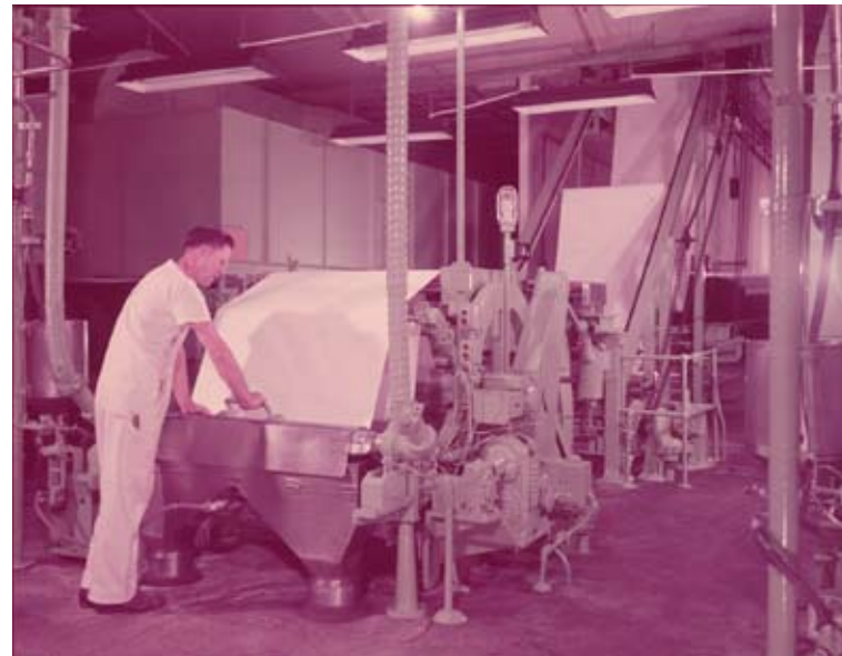
One of the Kodak baryta coaters showing an air knife coating process.
