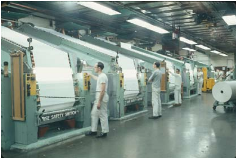
The winding sections of several Kodak baryta coaters (ca.1970) showing modernization of the operation. (Compare to image on p. 35 of the same process)
