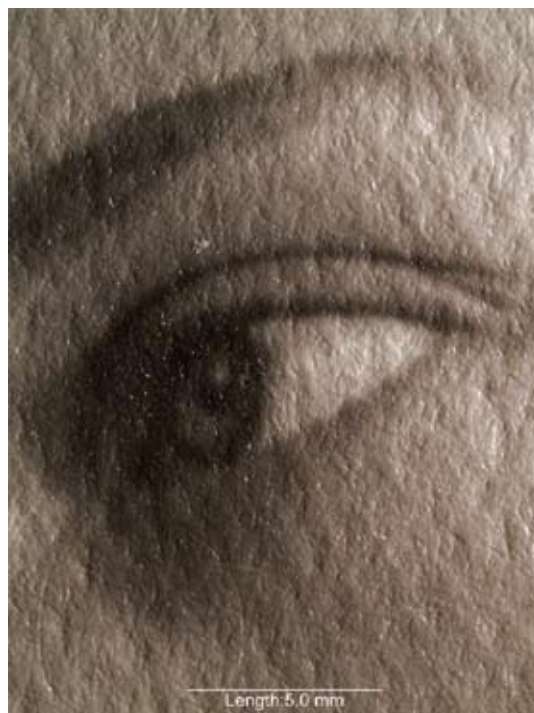
Kodak Kodabromide Grade R [Tweed] photographic paper sample and micrograph. "Photographic Papers Manufactured By Eastman Kodak Company" Rochester, Eastman Kodak Company., circa 1937 10.7 x 16.2 cm.
