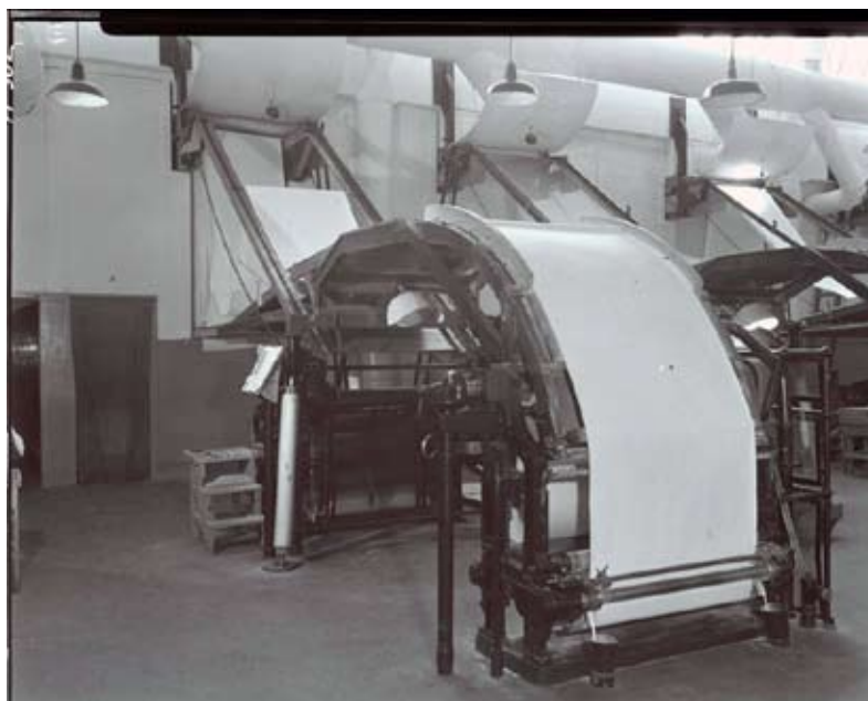
One of the Kodak baryta-coated paper winding mechanisms (1932).
