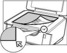
• When loading the Photo Index Sheet, place the front side down, and align the upper left corner of the sheet with the alignment mark on the lower right corner of the Platen Glass.
