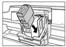
• Press firmly on the ink tank's tab until it locks into place.
