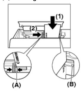
• Load the envelopes in the Auto Sheet Feeder with the short side down.
