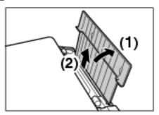
2 Place a stack of paper (print side up) in the Auto Sheet Feeder (1), and pinch the Paper Guide (A) and adjust it to the left side of the stack (2).
