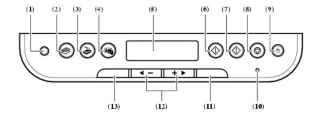
(1) [Photo Index Sheet]\* Button Switches the machine to Photo Index Sheet mode.
