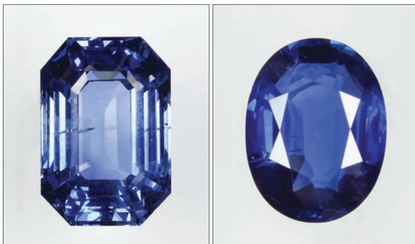
Figure 14: These unheated sapphires (left, 26 ct, and right, 11 ct) from Mogok, Myanmar, contain zircon inclusions that were age dated using LA-ICP-MS. Photos by Janine Meyer.
