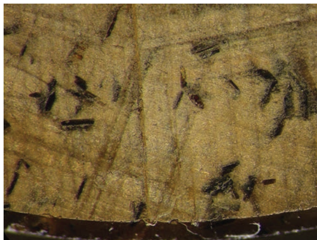
Figure 13: Hematite inclusions are seen here on the base of a black star sapphire cabochon. Photomicrograph by C. Williams; magnified 40×.
