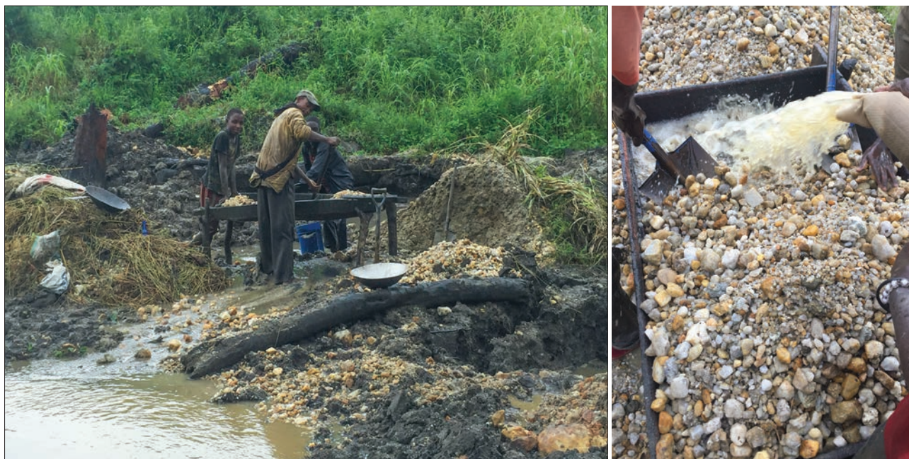
Figure 9: The mined material is washed with metal pans (left) or with pumped water (right), and then the garnets are hand-picked from the screens. Photos by Farooq Hashmi.
