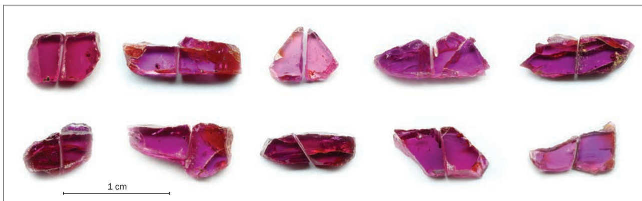
Figure 2: Ten rough ruby samples from Mozambique were sliced in half, and the right-hand portion of each sample was subjected to heating experiments (to 500 °C, and then to 600 °C), while the other half was kept for reference and colour comparison. Photo by T. Sripoonjan.
