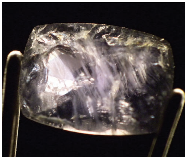
Figure 5: Fractures and wispy linear aggregates of microcrystalline chloritoid and/or chlorite form conspicuous inclusions in these sekaninaite gemstones (left magnified 5× and right 3×). The stone on the left also contains ferrogedrite (see arrow). Photomicrographs by R. Hanus.
