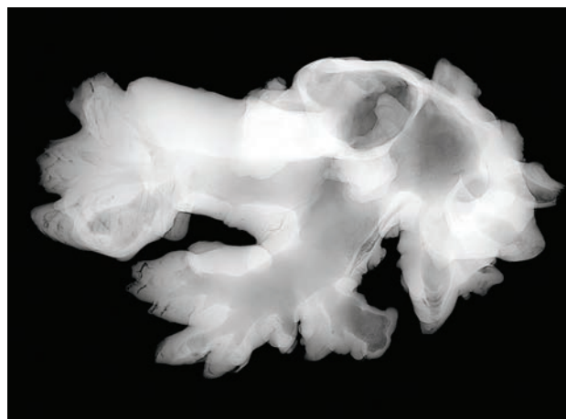
Figure 27: X-radiography of the biomineralized object (65 mm long) shows a dark-appearing void corresponding to a branch of coral that subsequently dissolved. Image by O. Segura.
