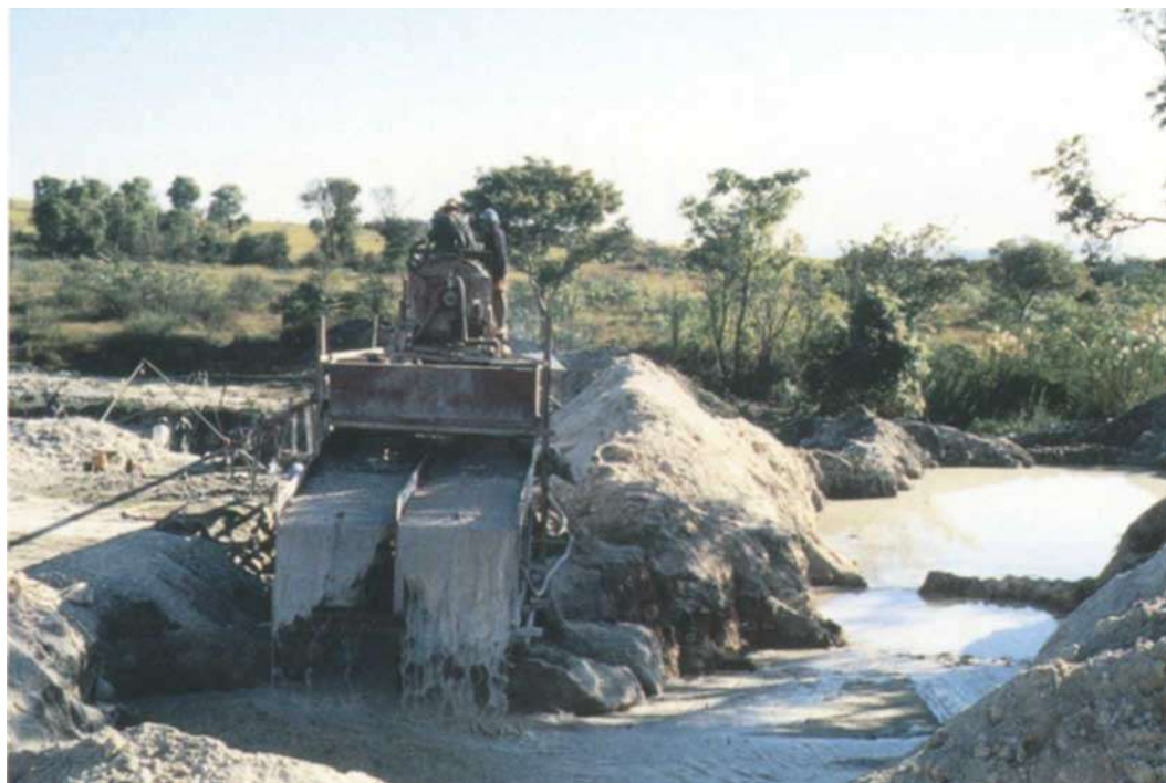
Fig. 6. The sapphire-containing gravel is treated by a jig in the working area of the companies Multicolour and Ste. Arc-en-Ciel Gem-Corp.
