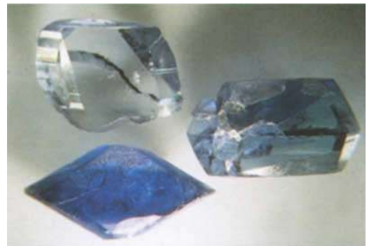
Fig. 13. Type III rough crystals showing different colour zoning. Magnification 2x.
