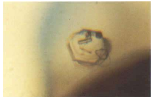
Fig. 10. Transparent, colourless birefringent mineral platelets (probably mica) are typical inclusions in the sapphires from south-eastern Madagascar. Immersion, transmitted light, 50x
