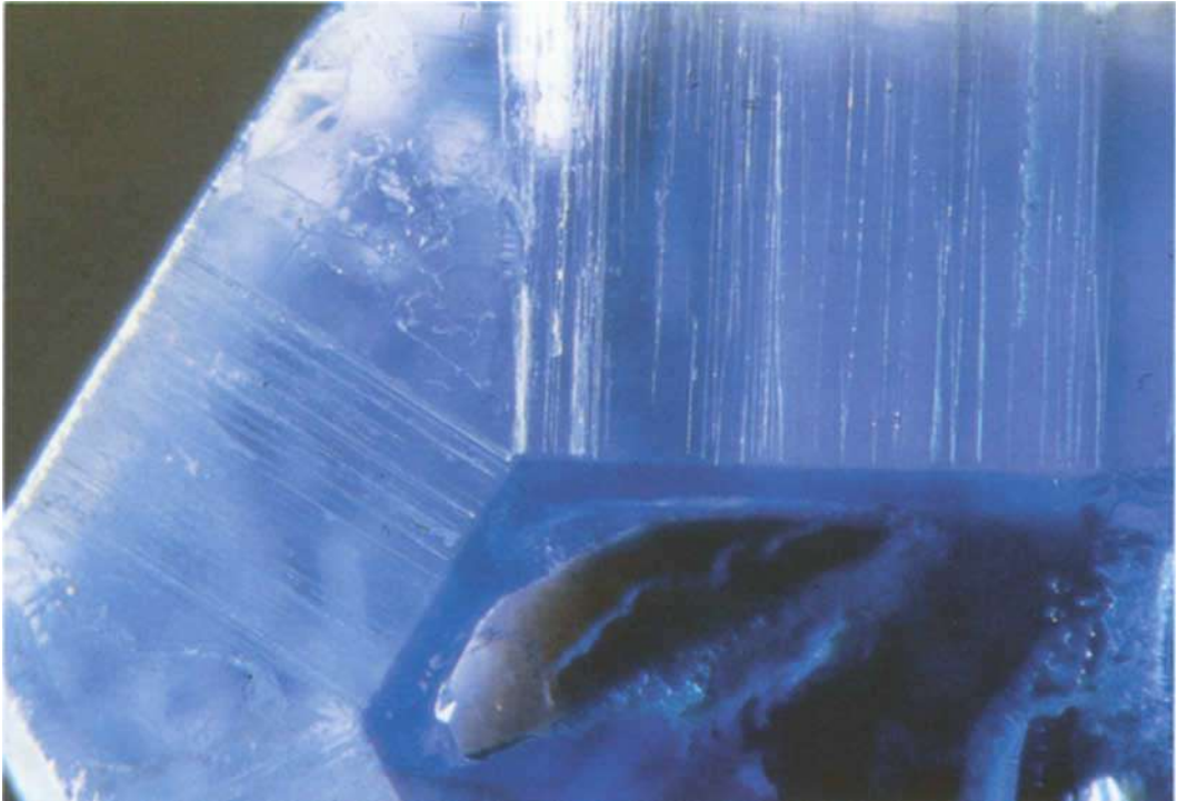
Fig. 12. Type II sapphire from Madagascar showing the dark blue core and lighter blue rim with white striations on the basal faces with an orientation perpendicular to the prismatic growth planes. View parallel to the c -axis. Magnification 4x.
