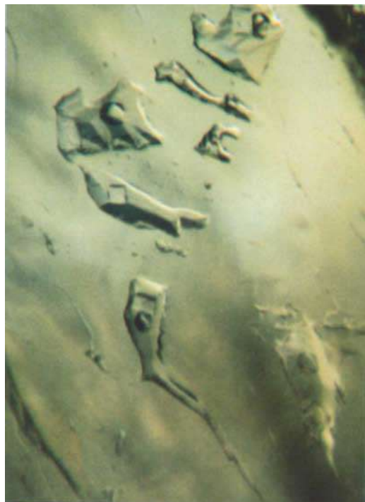
Fig. 2. Some of the numerous three-phase inclusions observed under the microscope. Magnification 60x.
