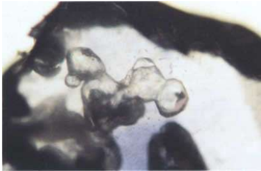
Fig. 9. Cluster of distinctly corroded, birefringent carbonate inclusions in front of a barely visible fingerprint-type healed crack. Immersion, transmitted light, 50x
