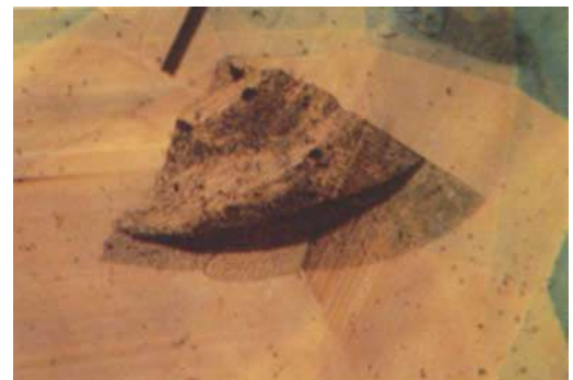
Fig. 25. Healed feather in sapphire from Madagascar. Immersion, magnification 50x.
