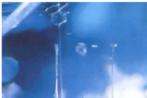
Fig. 27. Rounded apatite crystals with subsequent tubes in type II sapphires from Madagascar. Magnification 40x.
