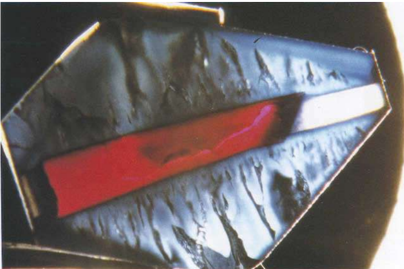
Figure 4: A section through a rough crystal of a synthetic sapphire produced by hydrothermal methods (TAIRUS), cut perpendicular to the c-axis. The seed crystals are composed of Verneuil synthetic ruby overgrown by synthetic 'hydrothermal' white sapphire. Note the blackish irregular tubes that emerge in a direction perpendicular to the seed crystal within the synthetic sapphire portion of the rough crystal. Fluid inclusions are trapped in these tubes. Terminating crystal faces are prisms (1120). Diameter 1 cm. Transmitted light.
