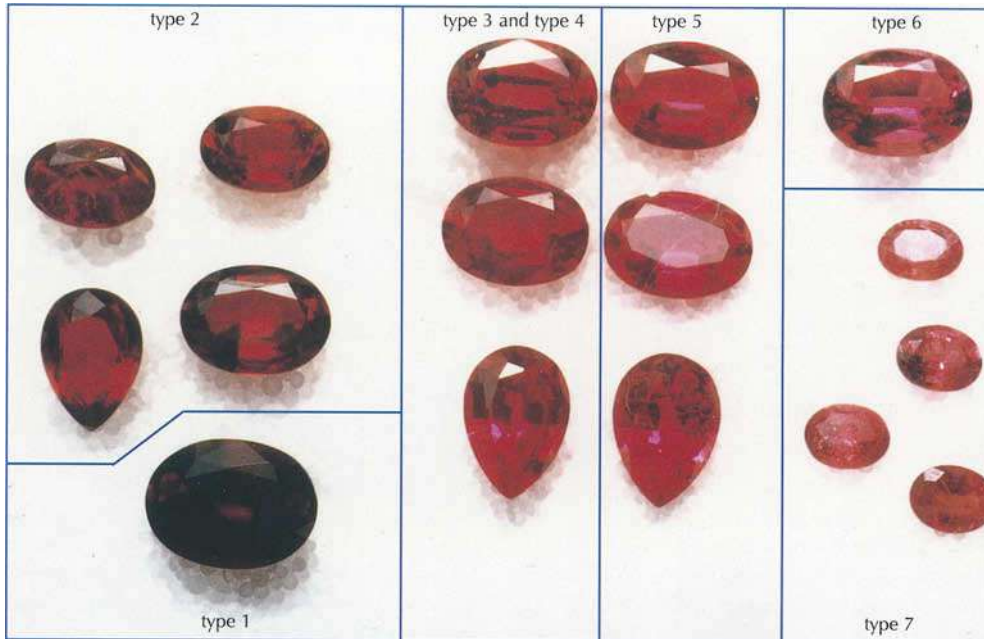
Figure 1: A set of faceted synthetic rubies produced by hydrothermal methods. From left to the right, different colour varieties are shown, including colours imitating Thai rubies (type 1 and type 2, Table I), Burmese rubies (type 3, 4 and 5) and Sri Lankan rubies (type 6 and 7). Sizes of rubies around 1 ct each, largest are 1.6 ct and smallest 0.2 ct. These products were created by TAIRUS (Novosibirsk, Russia) and purchased in Bangkok (Thailand).
