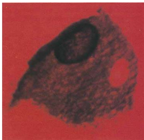
Figure 16b: Three-phase inclusion of Figure 16a as seen in immersion with crossed polarizers. The solid phase is more clearly visible because it is birefringent.
