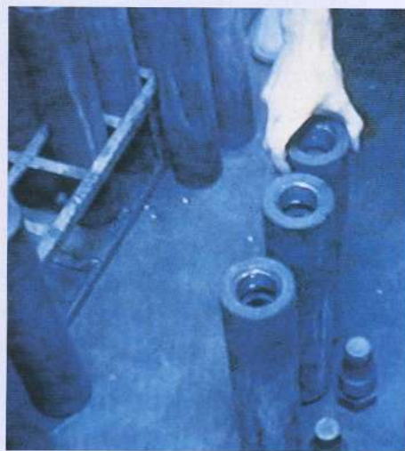
Figure 6a: The steel autoclave used for the production of the synthetic hydrothermal rubies in Novosibirsk (Siberia, Russia) in 1994. The weight of the autoclave is about 25 kg, the length is about 50 cm, the inner diameter is about 3–4 cm with slightly smaller estimated thickness of the steel walls. Inner liners of gold or platinum are fitted for production of Fe-free products, but their use is rare.
