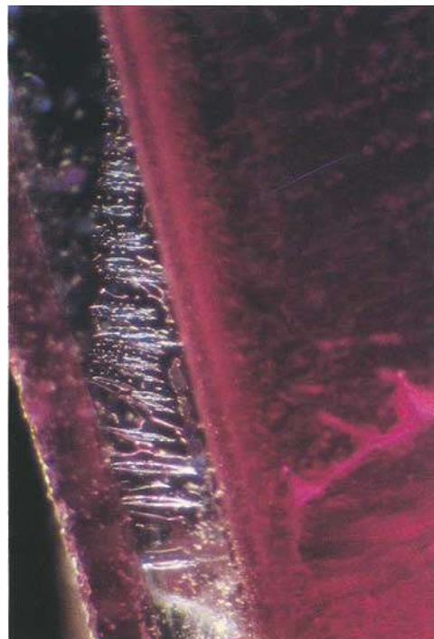
Figure 14b: Partially healed crack extending into the colourless synthetic sapphire seed (polished thick section). Reflected and transmitted light, fibre optic illumination. Length of shown portion of the crystal is 3 mm (type 4, Table I).
