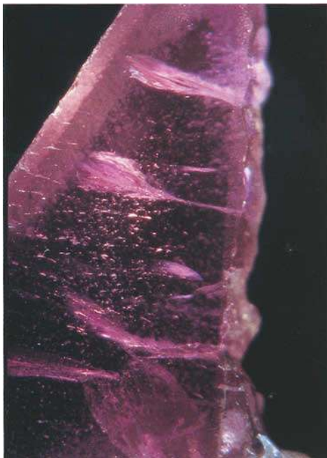
Figure 14a: Series of partially healed cracks in a rough ruby (polished thick section). Reflected and transmitted light, fibre optic illumination. Length of shown portion of the crystal is 5 mm (type 5, Table I).
