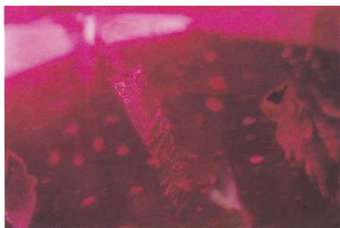
Figure 15: Large negative tubes found in faceted synthetic 'hydrothermal' ruby (type 5, Table III). Note the irregular walls of the tubes. Weight of ruby is 0.95 ct, magnification 100 x, transmitted and reflected light, fibre optic illumination.
