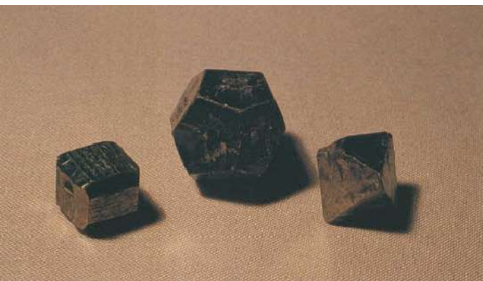
Figure 1: Group of pyrite crystals showing cube, pyritohedron and small octahedron (photograph by M. Hutchinson).
