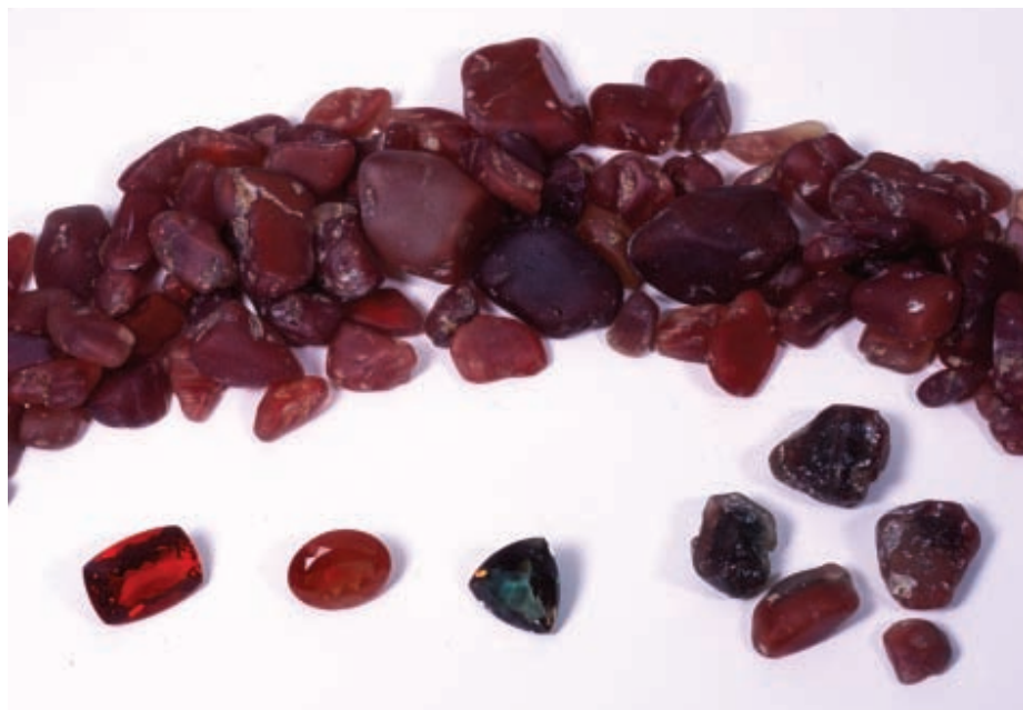
Figure 11: A pile of andesine rough (behind) collected from the Bainang mine in Tibet. These untreated rough materials of various colours (2.4–34.42 ct), are rounded and have a water-worn appearance. Parallel 'windows' were polished on two sides of each crystal to enable thorough examination. Cut samples (3.52–4.95 ct) in the foreground were supplied by M. P. Gem Corp., Japan. Photo by M. Kobayashi.
