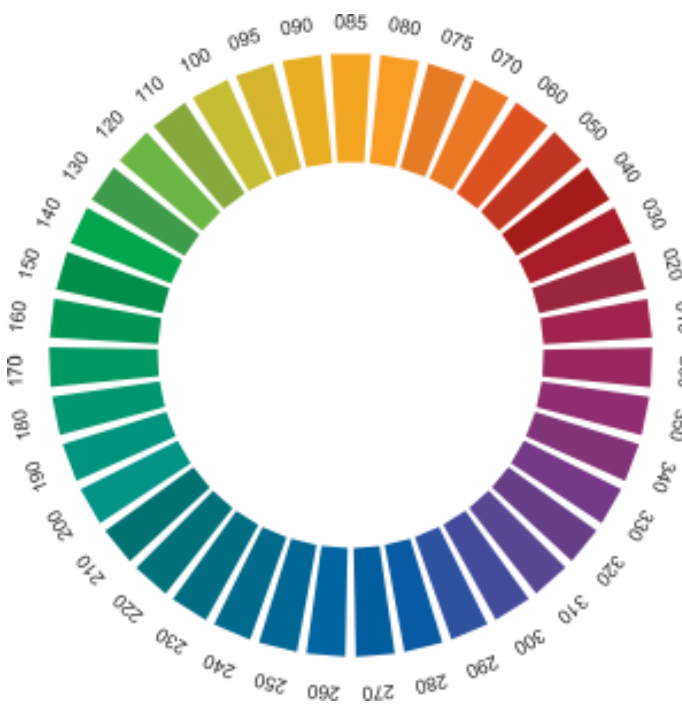
Figure 14: Hue circle (colour wheel) of CIELAB colour space representing examples of colours at different hue angles of the three-dimensional colour solid at high chroma and lightness 50. Copyright dtp studio Oldenburg and RAL gGmbH, Sankt Augustin, Germany (reproduced by permission).
