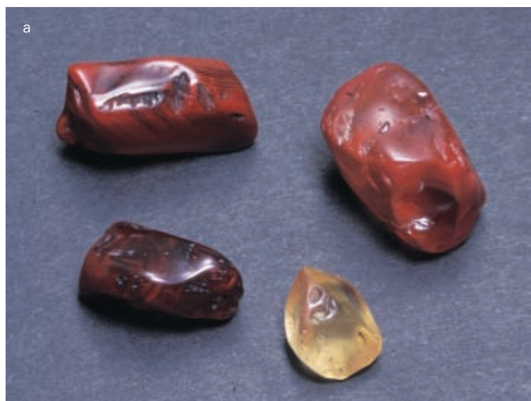
Figure 18: (a) Copper-diffused rough andesine crystals from China. (b-g) Sections of a copper-diffused andesine: an induced orange-red colour layer penetrates from the rim towards the core (b), but a colourless zone remains at the surface of the stone; red pipe-tubes, discontinuous lath-like hollow channels, a pipe and tube-like structure, irregular dislocations, milky turbid cloud, discoid fractures, and a recrystallized white residue can be seen in one treated stone. These features resemble Tibetan untreated andesine. Photos by A. Abduriyim; magnified 20-25x.
