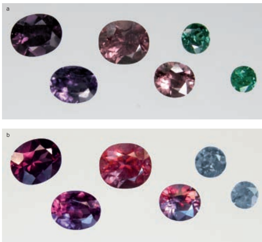
Figure 43 a,b: Colour-change garnets from Madagascar with hue angle differences between daylight (a) and incandescent light of below 20°; two samples of Group 4 (left), two of Group 7 (centre) and two of Group 2 (right) are pictured; diameter of the garnet in the lower right 3.9 mm, weight 0.28 ct.
