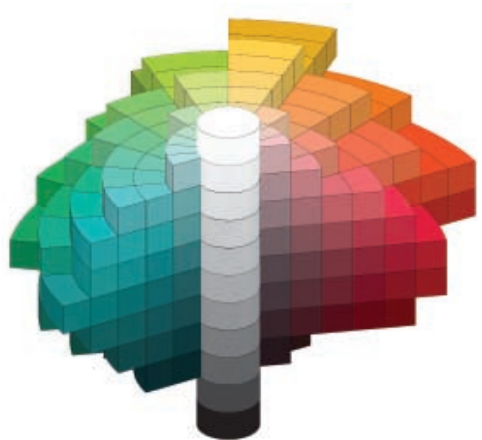
Figure 13: Model of the three-dimensional CIELAB colour space, model of the colour solid, section parallel to the non-chromatic (black to white) lightness axis. Copyright dtp studio Oldenburg and RAL gGmbH, Sankt Augustin, Germany (reproduced by permission).
