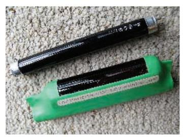
Figure 16: Small BLB 'black light' fluorescent LWUV tube (4 watt) above a 'germicidal' SWUV mercury based (4 watt) fluorescent tube fitted with a CoSO, solution filter and green sleeve.
