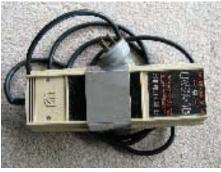
Figure 2: A combined LW and SWUV lamp UVSL-15 from UltraViolet Products (UVP).
