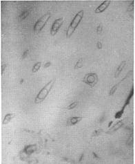
Liquid and gas filled inclusions in brazilianite. × 100. (<sup>\*</sup><sub>2</sub>" objective X10 ocular.)
