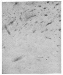
Liquid filled inclusions in brazilianite.  $\times$  20.  $(1\frac{1}{2}'' \text{ objective X6 ocular.})$
