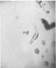
inclusions and a few larger cavities partly filled with liquid and a movable gas bubble.
