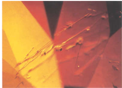
Fig. 4. Veil-like dislocations and small included crystals of undetermined nature were detected in two of the test samples. 50x. Photomicrograph by John I. Koivula © GIA
