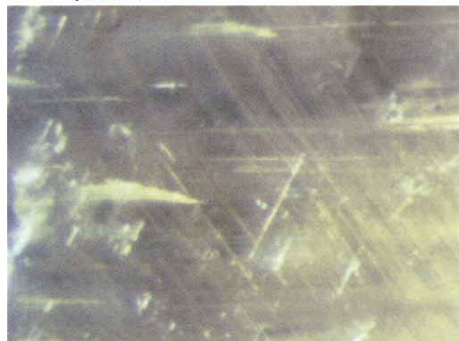
Fig. 10. Sample 17. Systems of parallel tubes and healing fissures cross this brownish-yellow zoisite from Lelatema District (Tanzania). 30x.
