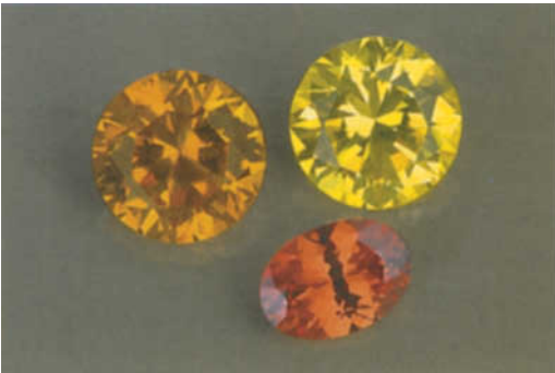
Fig. 2. These three gems (1.35 to 3.26ct), fashioned from single crystals of synthetic zincite, were the subjects of the current investigation. Photo by Maha DeMaggio © GIA
