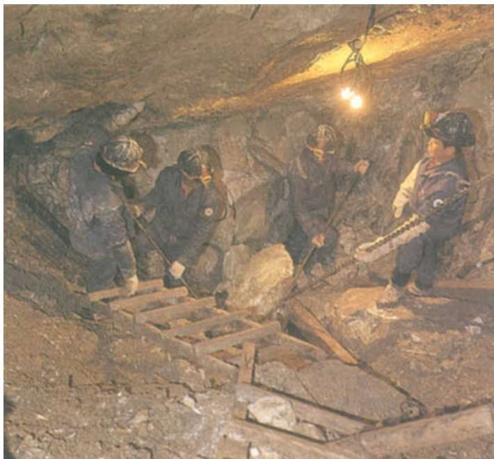
Fig. 3. Mine workers remove nephrite ore at the Daeil Mine, Chuncheon, Korea. The nephrite ore develops along the contact between the dolomite marble bed and the enclosing biotite schist.
