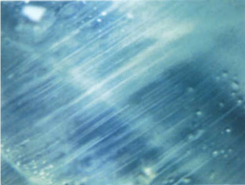
Fig. 4. Sample 4. In this aquamarine from Embu and Meru area (Kenya), the cat's-eye effect is caused by massed parallel, hair-like tubes. 20x.
