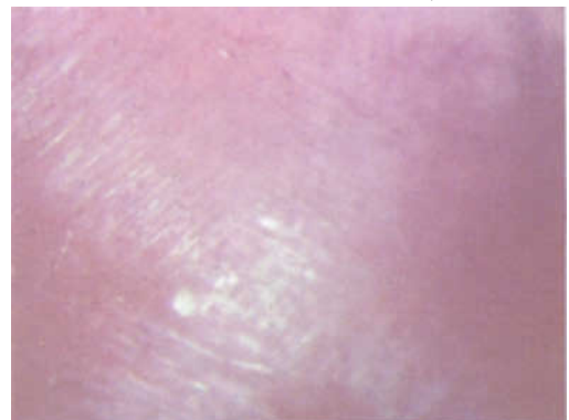
Fig. 7. Sample 10. In this ruby from Mt. Taita (Kenya), the crystallographically dictated arrangement of syngenetic rutile needles and lamellar structures cause the hazy asterism displayed by this cabochon. 10x.
