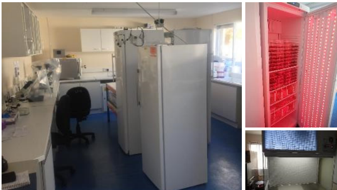
Figure 1. (A). Wet laboratory set-up used for spores release from gametophytes prior to the hatchery step, as well as the analysis and the quality control of seeded lines. Benches and an autoclave (visible at the back) were installed, with small equipment such as stereomicroscope (on the left). (B). Kelp gametophytes are kept under red light (12:12) at constant temperature ( 13^\circ\text{C} ) in incubators (two are visible in A). (C). A laminar flow has been installed to work under sterile conditions, in particular to avoid contamination of the samples by pests or potential pathogens.
