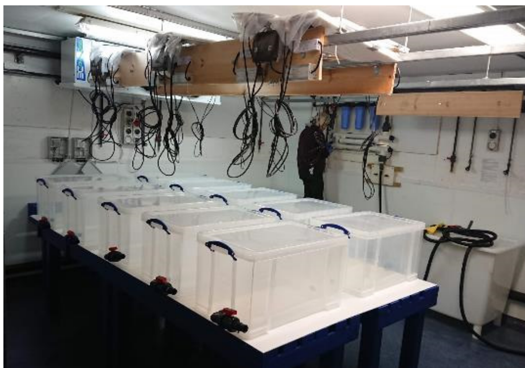
Figure 2. Hatchery setup with a capacity of 45km of twine lines (8000L), as of 2019. The principal components are the seawater supply with a sand-filtration system at 50, 20 and 1 µm (Fieder Filter Systems Ltd, UK) followed by 110W UV sterilisation (P2, Tropical Marine Centre Ltd, UK; see the blue structure on the rear wall). The tanks are independent from each other and easily washable, with waterproof LED lighting. The room was air-conditioned to maintain a constant temperature, a constant oxygenation intake for each tank.
