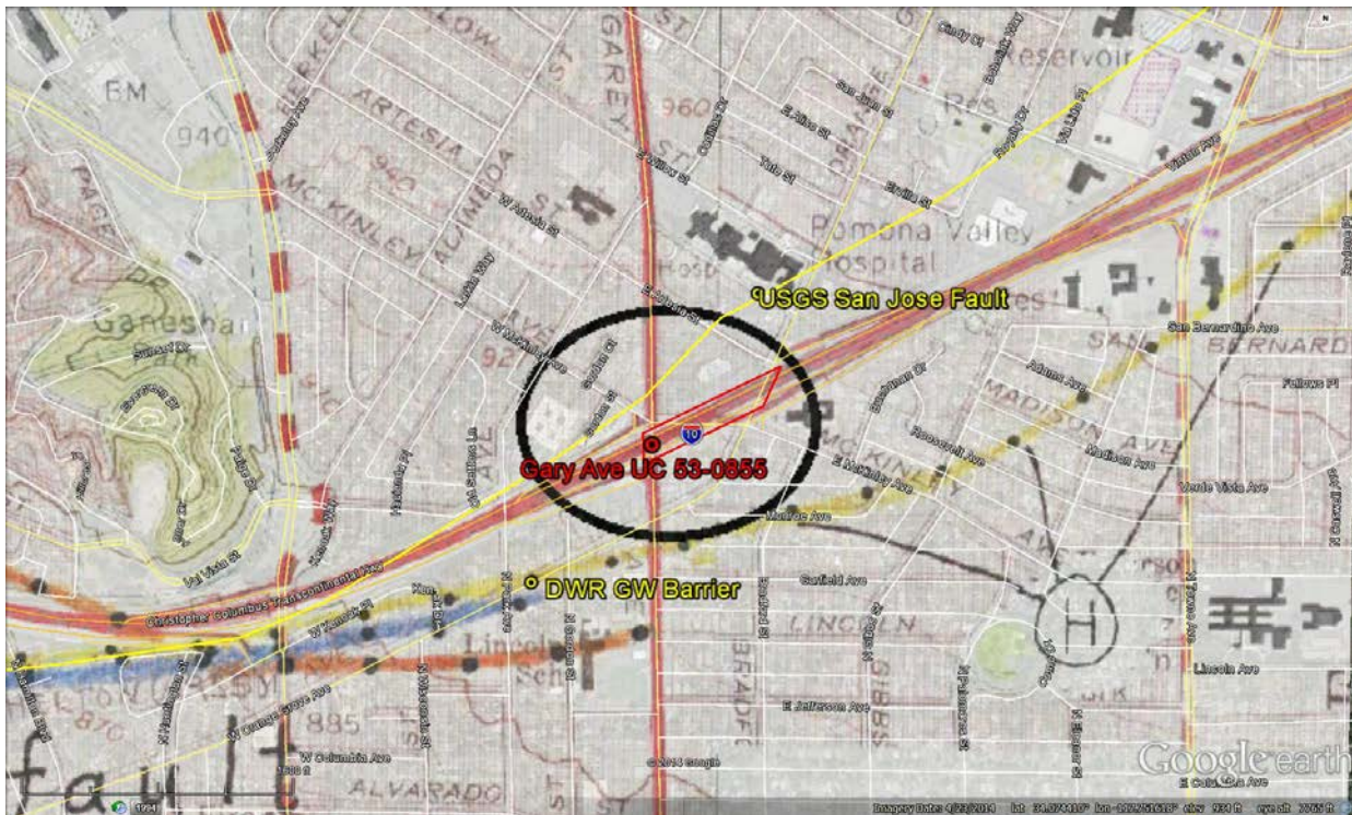
Figure 4: Image of Gary Avenue UC after CGS FER-68 (1977) and FER-68S (1978) after DWR (1970). Inferred groundwater barriers are black dotted and highlighted in yellow, blue and orange.
