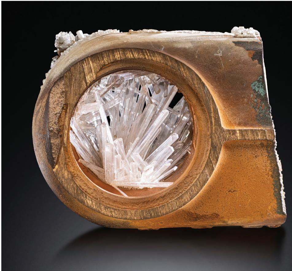
Figure 2. Recently deposited gypsum crystals in mining equipment.
