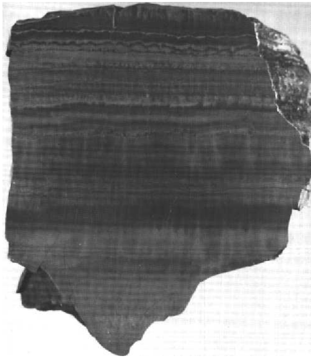
FIGURE 5—Banded, hard manganese oxides (psilomelane). Material of this type has been found to be dominantly hollandite with intergrown cryptomelane and coronadite. Sample is 6 cm wide.
