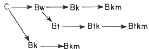
FIGURE 2—Parent material (C), with continued addition of aerosols to a stable geomorphic surface, transforms to cambic (Bw) to calcic (Bk) to petrocalcic (Bkm) horizons, or from cambic (Bw) to argillic (Bt) to argillic overprinted with calcic (Btk) to petrocalcic (Btkm) horizons, or directly to calcic (Bk) to petrocalcic (Bkm) horizons.
