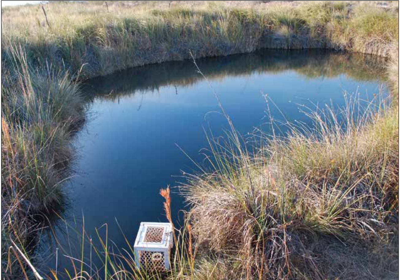
Figure 13. Example of a spring pool instrumented with a data logger. The white cage near the bottom of the photograph is a protective measure to prevent the instrument from being removed from the piezometer.
