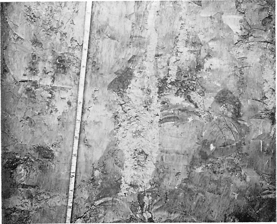
Figure 2.—Wall of Eliza Clark School test pit 15-16 feet below surface showing vertical silt-filled crack in the clay.
