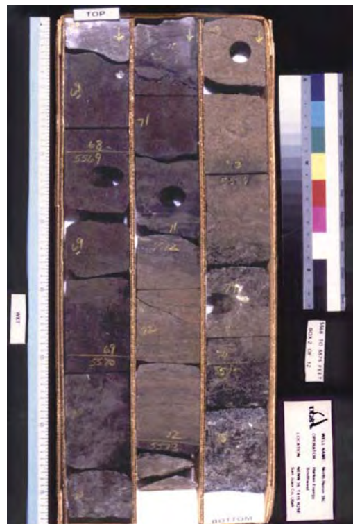
Figure 3-17. Core photograph of the highly dolomitized, oil-saturated calcarenite section of the North Heron No. 35-C well, Heron North field.
