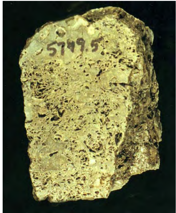
Figure 4-5. Phylloid-algal bafflestone in core of the producing oil reservoir rock from Mule field, San Juan County, Utah.
