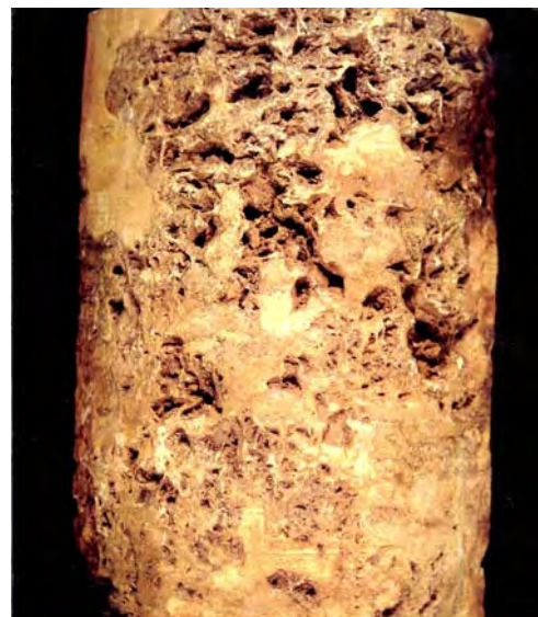
Figure 3-12. Core surface view of highly productive, dolomitized, phylloid-algal plate bafflestone from the Mule No. 31-M well, Mule field (see figure 3-11 for seismic line through well). Note good visual shelter porosity. Core diameter = 3.5 inches (8.9 cm).
