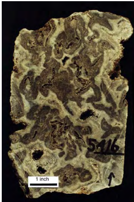
Figure 3-20. Slabbed core segments from 5,415.5 to 5,416.1 feet (1,650.6-1,650.8 m) of the Blue Hogan No. 1-J-1 well showing the typical pattern of marine cementation within the well-lithified “wall” complex.
