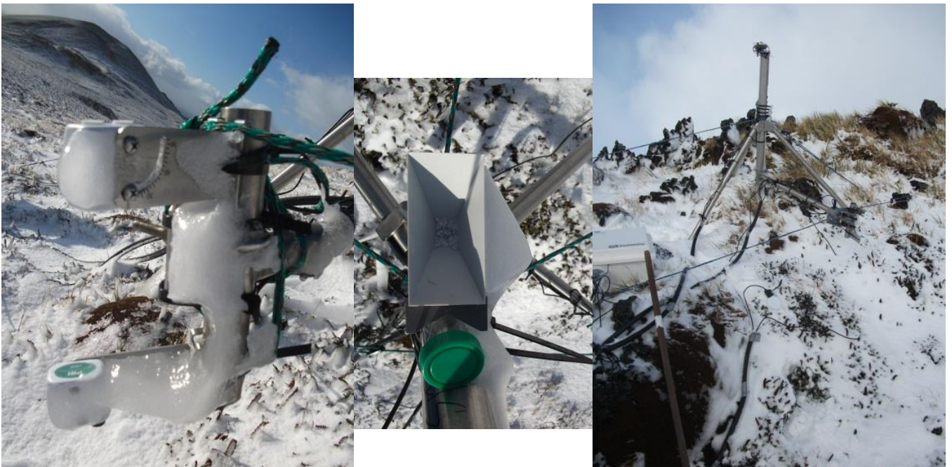
From Left: Sensors measuring incoming and reflected wavebands; Rain gauge (measuring one of the many environmental factors); The equipment battling with snow and ice
