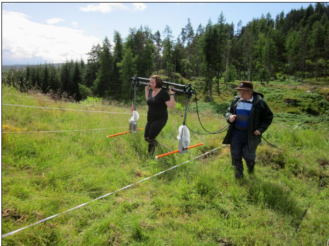
Figure 16: Jackie Hoyt and Dr. Nicholas Dixon maneuvering the 80 MHz MLF GPR antenna and armored data cable along Line 15 (reproduced with permission of the photographer, Ervan Garrison).
