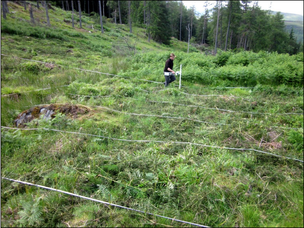
Figure 14: The author operating a Bartington Grad-601 fluxgate gradiometer along line 2 in grid 5 (reproduced with permission of the photographer, Ervan Garrison).
