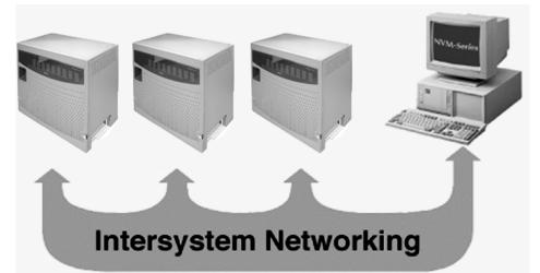
Use the built in networking feature to integrate multiple phone systems into a single "virtual" communications system. Interconnected with ISDN PRI or BRI or VoIP, each phone system becomes a node on the network that can communicate with any other phone system node.
