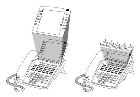
An extension user can chain dial with One-Touch Keys. For example, a user can store the number for a company's Automated Attendant in key 1 and employee extension numbers in keys 2-5. The user presses key 1 to call the company, then one of keys 2-5 to ring the employee to which they want to speak.
