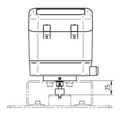
NAMUR Mounting Pad: Rotary positioners all utilize the same NAMUR compliant mounting pad if used with a GF pneumatic actuator. An operator can see the rotary position sensor for optical position indication.
