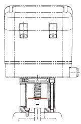
With Optical Indicator: Linear positions can utilize a GF DIASTAR Valve specific mounting pad that utilizes an orange colored disc on the sensing pin and a viewing window on the mounting pad to provide the user with an optical indicator.
