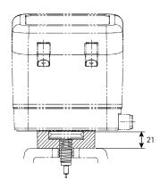
Without Optical Indicator: Linear positions can utilize a GF DIASTAR Valve specific mounting pad that lowers the overall footprint of the assembly but does not allow the user to see the position of the valve.
