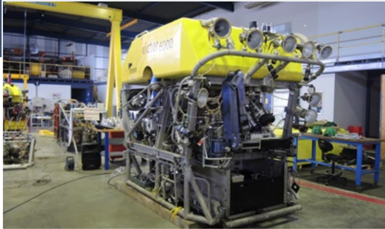
Victor 6000 véhicule sous-marin téléguidé (ROV – Remotely Operated Vehicle). veicolo robotico filoguidato (ROV – Remotely Operated Vehicle).
