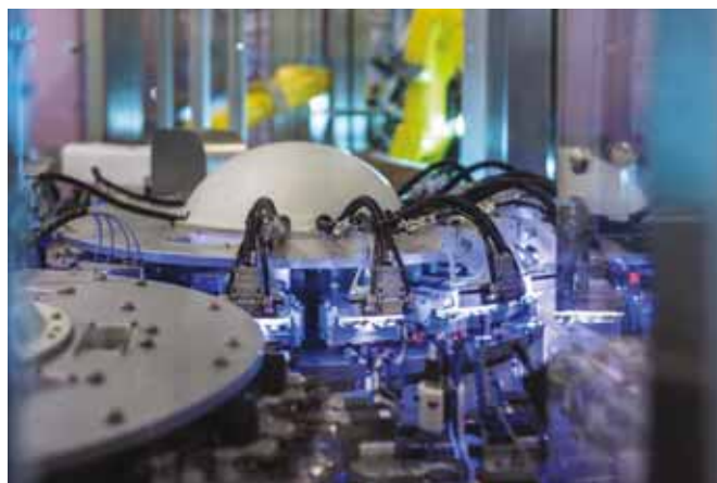
Needle assembly machine with LED-light curing system to improve glue polymerization
