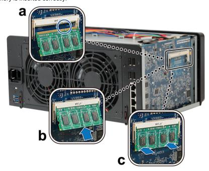
Important: Hold the memory module by its edges, and do not touch the gold connectors.
