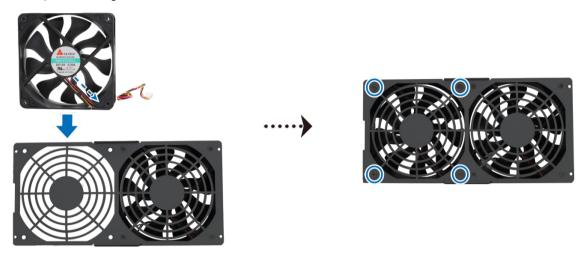
**b** Connect the 2 fan cables to the connectors located near the bottom of the fan socket, and then replace the fan panel.
