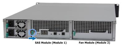
3 Pull out the SAS / fan module from the expansion unit.
