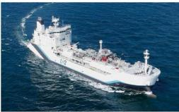
Suiso Frontier liquefied hydrogen carrier
