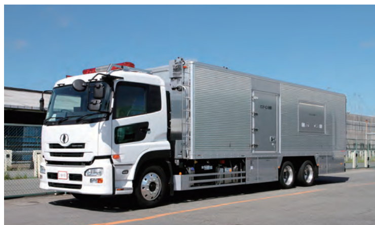
Fig. 5 Mobile power unit
