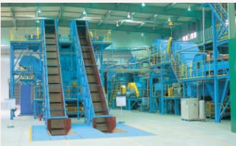
RPF (fuel derived from solidified waste paper and plastic) production facilities
