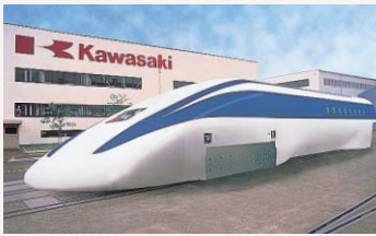
Magnetically levitated linear motor-driven high-speed train (for JR)
