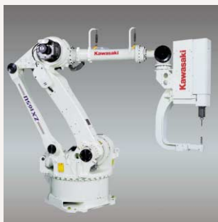
Typical system configuration that combines the special gun and an articulated robot
