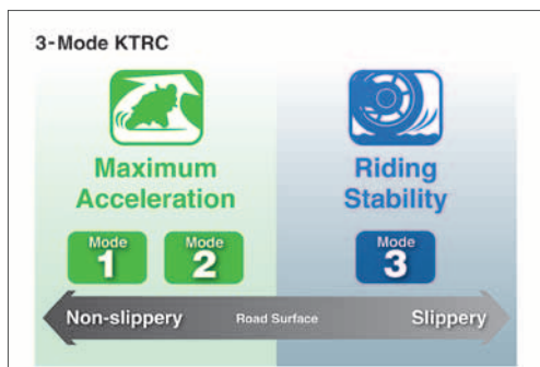
Operational modes of Kawasaki TRaction Control
