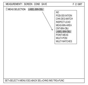
Press the ESC key to return to the OBJECT TYPE COND (menu tree) screen, and select the "MEAS CND" item shown under "MEAS01 (LABEL-BIN-OBJ)" to go to the "MEA-CND" screen.
