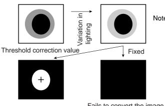
Note: In order to use the THRESHOLD-ADJ(threshold adjustment function), the monitor brightness functions must be selected to measure variations in lighting. If you don't select the monitor brightness function, a LIGHT LVL NOT SET (correcting binary value: monitor illumination not selected) error will occur.
