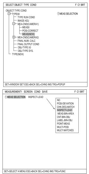
Press the ESC key to return to the "OBJECT TYPE COND" (menu tree) screen, and select the "MEAS CND" item shown under "MEAS01 (INSPECT-LEAD)" to go to the "MEAS CND" screen. ⇒ For details, see "Chapter 8: Setting Examples Using the Menu Tree" in Introduction and Hardware.
