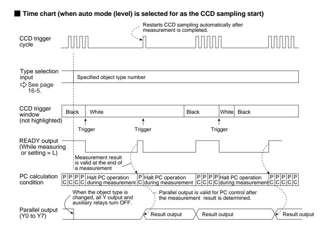
(10) Measurement start input = CCD trigger, start sampling = auto, object type change = general purpose serial, result output = general purpose serial/parallel
