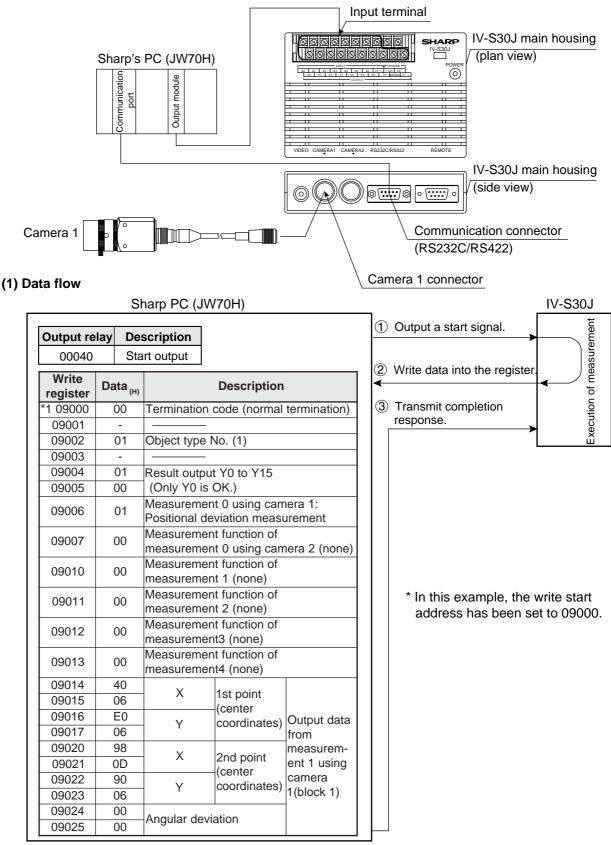
Note 1: The PC must be write enabled. A Mitsubishi, OMRON, or Yokogawa PC will operate in the same manner, but use different PC register and relay addresses.
