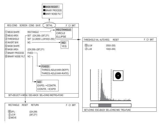
1. Specify a measurement area smaller than the mask area and specify the binary conditions.
