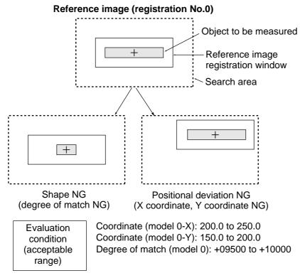
(2) Output conditions and ladder circuit for measurement 0 using camera 1 When the X coordinate, Y coordinate and degree of match are within acceptable ranges, the auxiliary relay C000 is turned ON.
