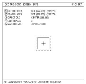
Then, press the left or right arrow key to move the cursor to the next five digits, which are the upper limit. Adjust this number the same way.
