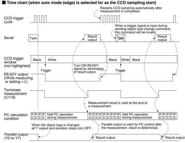
Note: Result output; The data in the block No., set in item "⑤SET SERIAL BLOCK" on the "OBJ-TYPE I/O" screen, will be transmitted to the personal computer.
