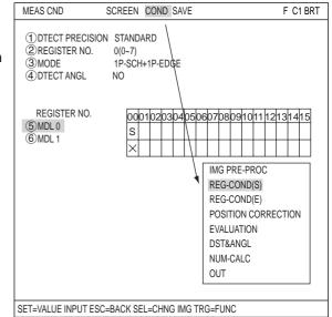
3) On the menu tree, move the cursor to the "MEAS CND" item, and press the right arrow key. The sub menu which contains the "REG-COND(S)" and "REG-COND(E)" items will appear. Move the cursor to either of these items and press the SET key.
