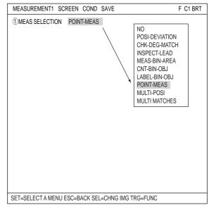
Press the ESC key to return to the "OBJECT TYPE COND" (menu tree) screen, and select the "MEAS CND" item shown under "MEAS01 (POINT-MEAS)" to go to the "MEA-CND" screen.
