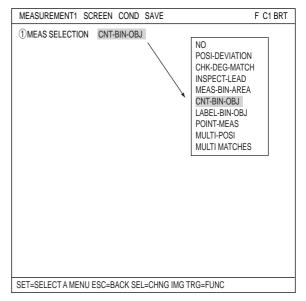
Press the ESC key to return to the OBJECT TYPE COND (menu tree) screen, and select the "MEAS CND" item shown under "MEAS01 (CNT-BIN-OBJ)" to go to the MEA-CND screen.
