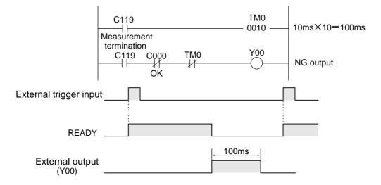
(3) An example of a circuit that can output a signal when the IV-S30 is operating normally.
