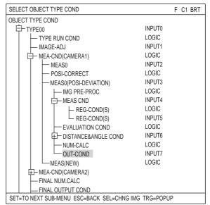
2. On the screen used for selecting the measurement program, or on the screens used for setting the measurement conditions or the register conditions, press the TRG/BRT key to move the cursor to the upper function menu. Then, move the cursor to the "COND" and press the SET key. Select "OUT" from the popup menu.
