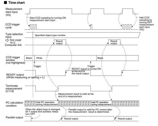
Note: Result output: The data in the block No., set in item "⑤SET SERIAL BLOCK" on the "OBJ-TYPE I/O" screen, will be transmitted to the personal computer. □ See page 16-23. (8) Measurement start input = CCD trigger, start sampling, object type change = general purpose serial, result output = general purpose serial/parallel
