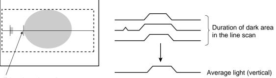
Edge detection point (with artifact processing: enabled)
