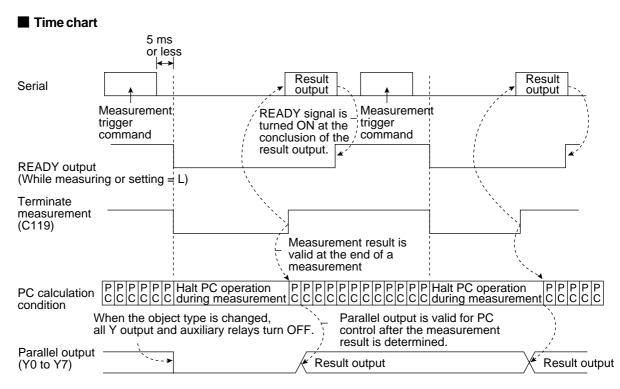
(5) Measurement start input = CCD trigger, start sampling = parallel, object type change = parallel, result output = parallel
