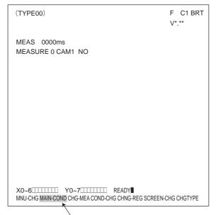
Move the cursor to the "MAIN COND" item using the left and right arrow keys and press the SET key.
