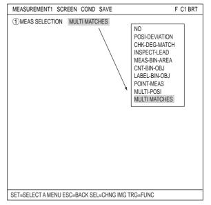
Press the ESC key to return to the "OBJECT TYPE COND" (menu tree) screen, and select the "MEAS CND" item shown under "MEAS01 (MULTI MATCHES)" to go to the "MEAS CND" screen.
