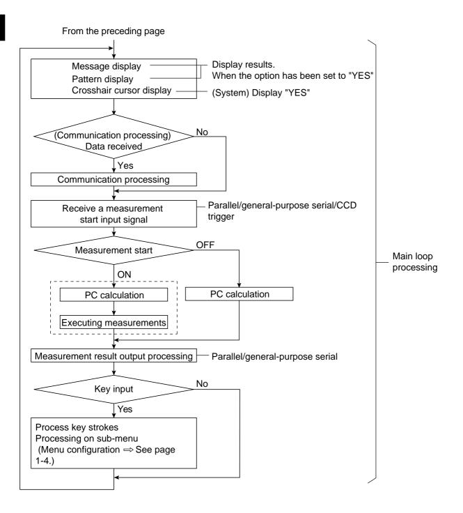
[2] Operation flow after the measurement start input is turned ON.
