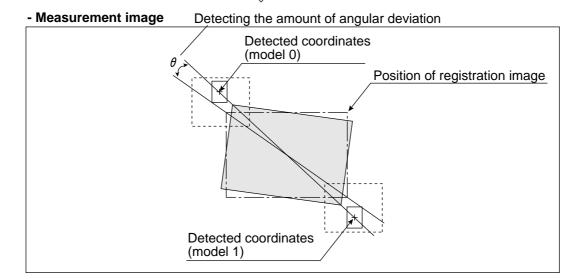
2. Performing measurement 1 to 4 (of distance and angle measurement) on an image that has been rotated around its center by the amount of angular deviation detected in step 1.
