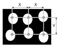
Enter 002 (vertical) · 003 (horizontal) in item "⑥BLOCK ARRANGEMENT," and enter the vertical (Y) and horizontal (X) intervals in item "⑦BLOCK SPACING." Then select item "⑧STORE BLOCK OF PTS" to store the settings for the block.
