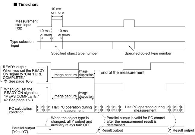
Note: When the READY signal is turned ON, the measurement start input will be enabled. To detect the end of the measurement, you have to create a ladder circuit pointing at the Y output for auxiliary relay C119 (end of the measurement).
