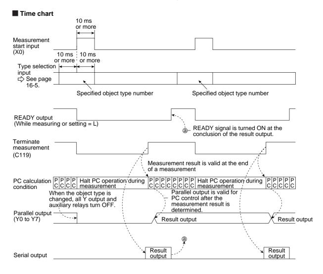
Note - Result output: The data to be sent to the personal computer will be response of general-purpose serial command (code 11<sub>(H)</sub>).
