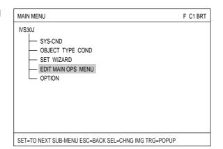
(3) Now the operation screen will appear. Select a block of text you want to edit using the up, down, left, and right arrow keys, and press the SET key. A pop up menu will appear and you can select from move, enlarge, reduce, and hide. (In this example, the block of text "OK" is selected.)
