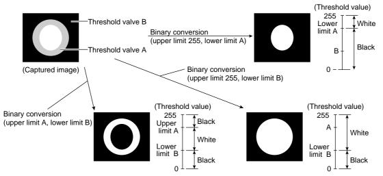
Setting the threshold value automatically The binary threshold value can be set automatically.
