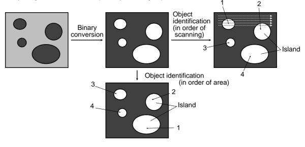
Measurement programs which are affected by these settings Object counting by binary conversion, object identification by binary conversion
