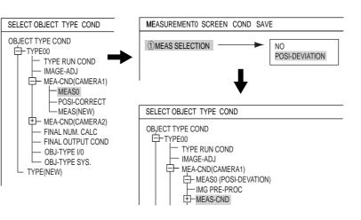
Note: "POSI-DEVIATION" (positional deviation) measurement can be specified in the "MEAS0" (measurement 0) and "MEAS1" (measurement 1) to "MEAS4" (measurement 4) functions. If you choose "MEAS(NEW)," the smallest available measurement number will be chosen automatically ("MEAS1" to "MEAS4").
