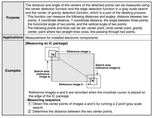
For details about measuring the distance between two points, X coordinate distance, and Y coordinate distance manually, see the MANL-MEAS (manual measurement) section (page 2-13) for the crosshair cursor display.
