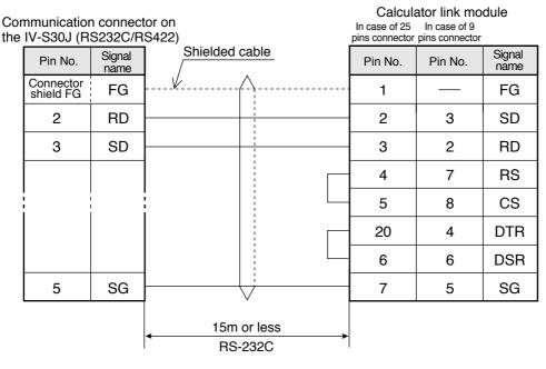
Note: Jumper the RS, CS, DR and CD lines. Do not jumper the SG.
