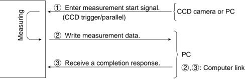
The block of measurement data to be written from the IV-S30J to the PC, in step ②, can be specified on the "OBJ-TYPE I/O" screen.
