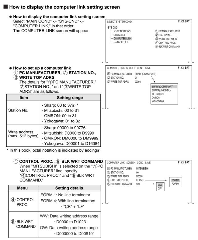
See "Chapter 18: Computer Link" for applicable models made by these manufacturers. Note 1: Use an even address as the write start address.
