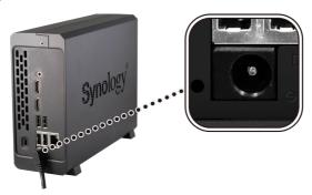
2 Connect one end of the LAN cable to VS240HD and the other end to your switch/router/hub.
