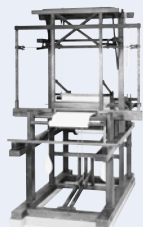
Sakichi's first invention: The Toyoda wooden hand loom (photo provided by the Toyota Commemorative Museum of Industry and Technology)
