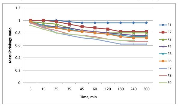
Figure 4 : Effect of NaCl concentration and immersion time on shrinkage ratio (SR)
