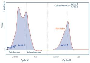
Fig 30 Idealized force-deformation curve for textural parameters
