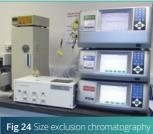
Fig 24 Size exclusion chromatograph with multi-angle light scattering equipment
